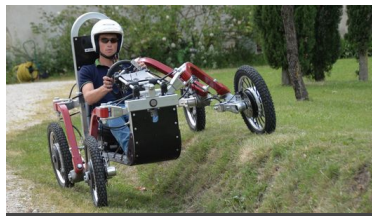
Swincar tilting 4-wheel-drive "spider car" makes light work of bizarre terrain
